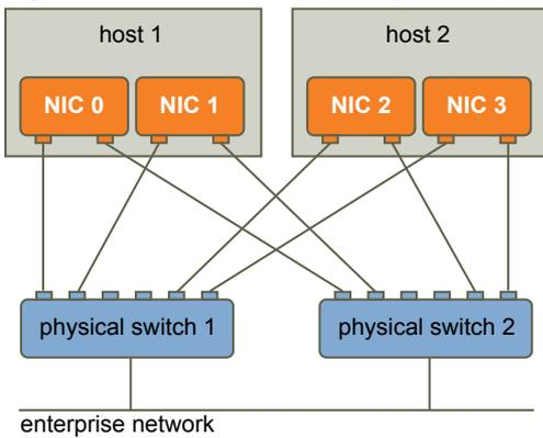
**Figure 1-4.** Network Redundancy in a VSA Cluster with 3 Members
